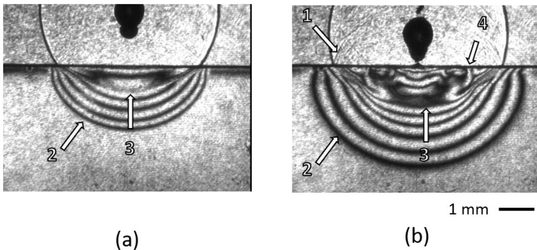
**Figure 2:** Photoelastic image of laser-excited acoustic waves in the solid. Delay time: 1500 ns. The laser came from above. The focal point is located (a) 1.1 mm above the target and (b) 0.6 mm above the target. The acoustic waves are numbered as 1: reflected wave, 2: P-wave, 3: S-wave. 4: Scholte wave.
