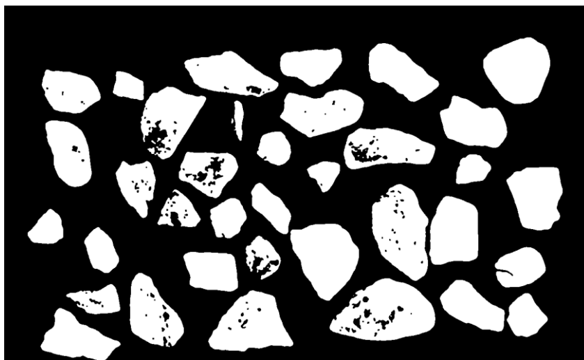
Figure 3.2. The result of the image thresholding process
