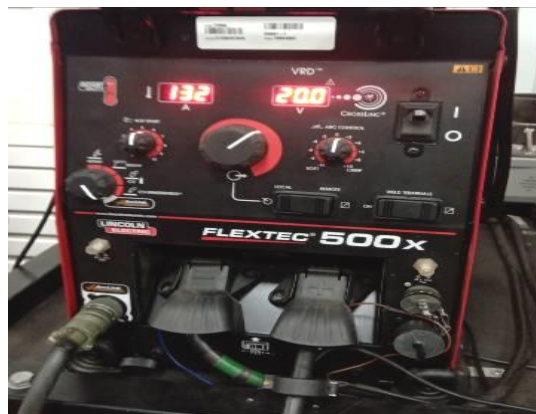
Fig. 2. PLEXTEC® 500x welding machine and welding process parameters.
